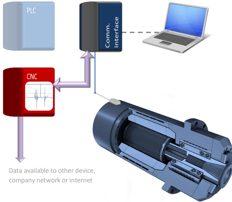
The communication interface allows bidirectional data exchange between the sensor and the machine CNC.
